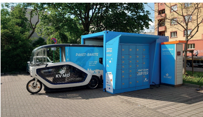
Figure 1: Example of system components (cargo bike, static parcel station, battery-swap station, micro depot)
